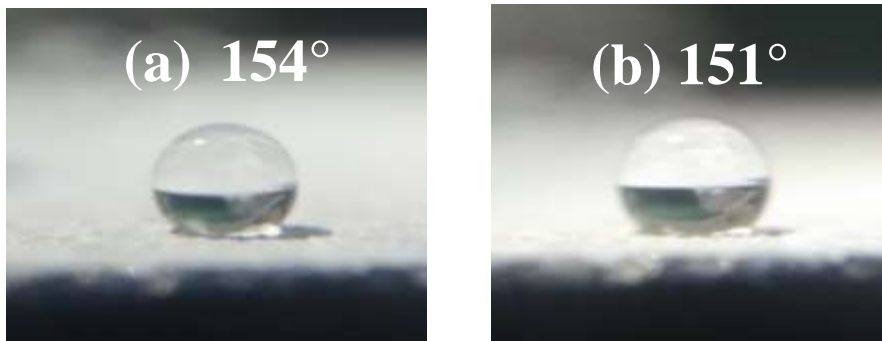
Fig. 5 Water contact angle (WCA) on (a) metal and (b) glass substrate
